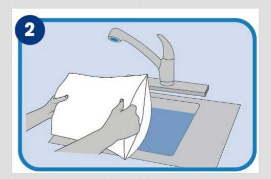
Energise your FloodSax®. This can be done by soaking the FloodSax® with water until they are fully expanded. This should take 2 to 3 minutes.
