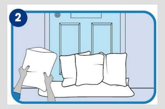
And then build a wall on top by vertically overlapping the other energised FloodSax®.
