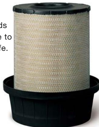
Hot melt bonding ensures proper alignment and protection of pleats throughout filter life. Corrosion resistant, closed metal plates with durable mag-grip handles ensure easy installation and service. Fleetguard gasket designs and compounds are hermetically sealed for each application to ensure reliable fit throughout the filter's service life.
